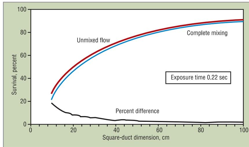
FIGURE 4. Survival of E. coli under mixed flow and unmixed flow in square ducts of increasing dimension.
